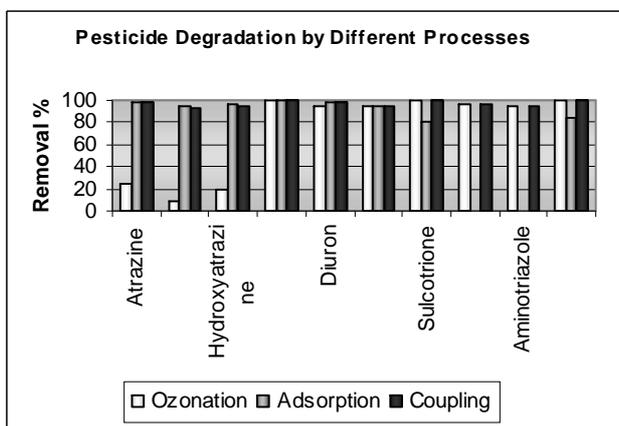
**Figure 1 Pesticide removal from membrane concentrates by ozonation, adsorption and combined processes** (TOC= 16.11 mg/L, COD= 33.3 mg/L CPAC= 30 mg/L, CO<sub>3</sub>= 3 mg/L, tc= 10 min)
