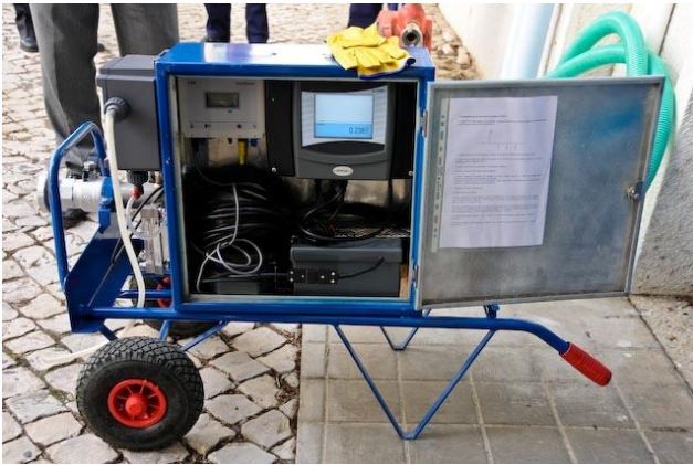
Figure 2 Trailer-mounted RPM measuring equipment developed by EPAL
