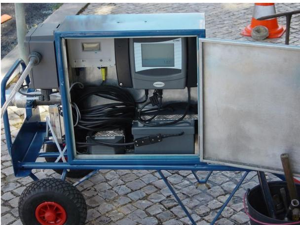
**Equipment developed for RPM measurements in the Lisbon Case Study**
