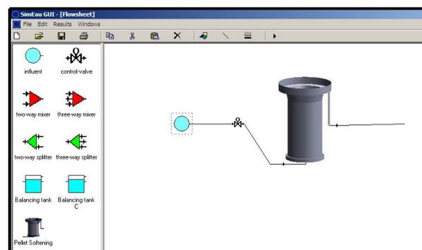
The European Water Treatment Simulator: Example of a flowsheet for a pellet softening plant
