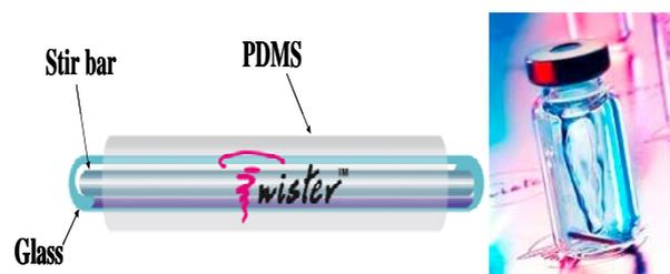
Figure 1 SBSE: The Twister™ support and its application
