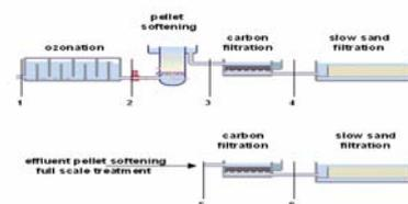
**Figure 2 Overview of pilot plant and sampling points**
