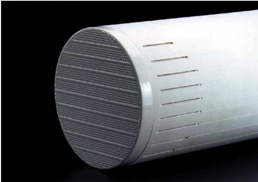
Fig. 2.2: Example for a monolith type ceramic membrane module 25 m 2 membrane area, 2.000 channels with 2.5 mm in diameter (photo: NGK)
