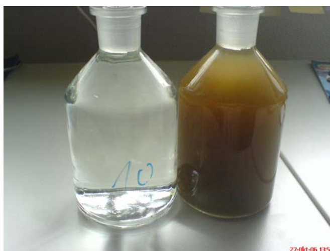
Fig. 4.4: Samples of feed (right) and filtrate (left) of the SiC-membrane
