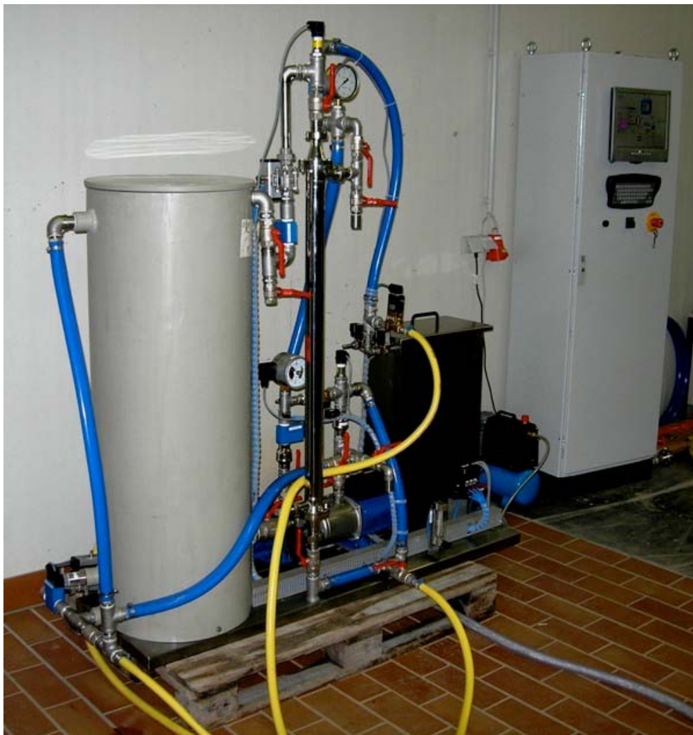
Fig. 3.1: Pilot plant for ceramic membrane filtration (left to the right: storage tank, membrane housing, filtrate tank, visualized stored program control)
