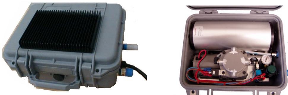
Figure 4: The compressor unit for field use. Left: exterior view. Right: view of internal parts of the unit.
