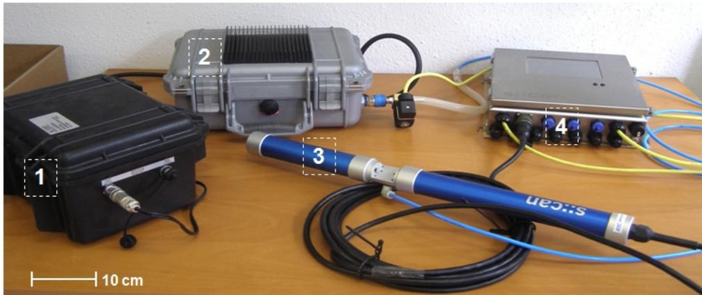
Figure 5: All components of the portable station assembled. From left to right: (1) weather proof battery pack, (2) weather proof compressor unit, (3) spectro::lyser™ spectrometer probe and (4) con::stat controller.
