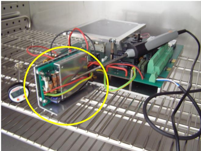
Figure 2: Temperature testing of the DC power supply in a climate control chamber.
